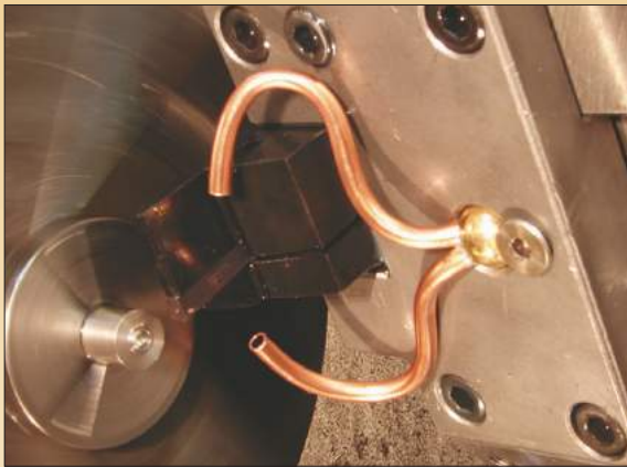
TwinPop nozzle shown installed in lathe turret.
