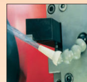
TYPE 2 OddBall attached to 1/4" Snap-Loc** hose.
