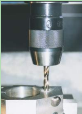
1 Drill coolant passage, leaving reaming allowance.
