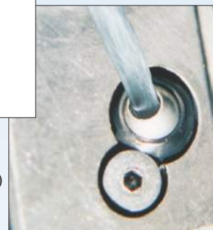
BlackEye installed on quick change turning tool.
