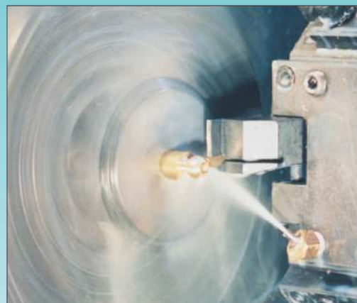
PressureMax nozzle shown in use on CNC turning center. High velocity coolant stream prolongs tool life and aids chip control.
