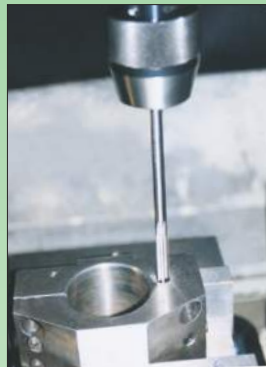
2 Ream hole to nominal size -0 \text{ } +.002\text{'}
